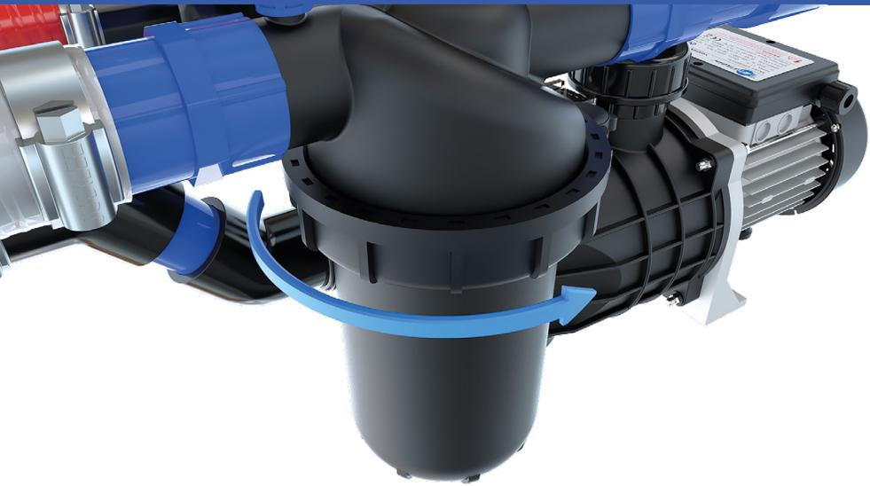
The water pump has a basket filter which catches larger debris. The secondary in-line filter has a fine mesh filter to remove smaller debris and organic matter. Both filters should be checked and cleaned when the system is empty, ideally when performing a nutrient change.
